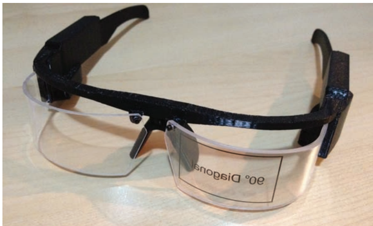
6. iOptik off axis projection with transfective diffuser 90° field eyewear model.
